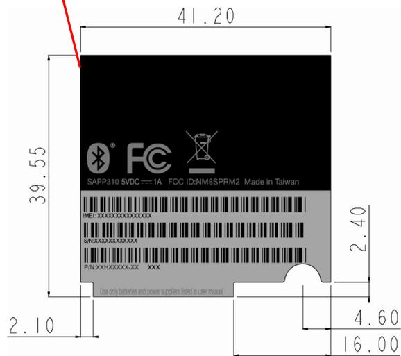
**NOTE: label on internal PCB board, not on back cover**
