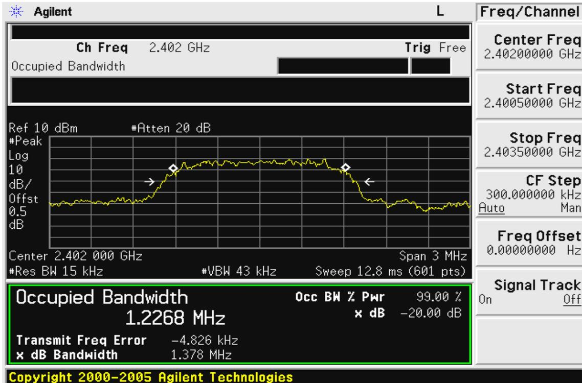
**20dB Band Width Test Data CH-Mid (EDR mode)**
