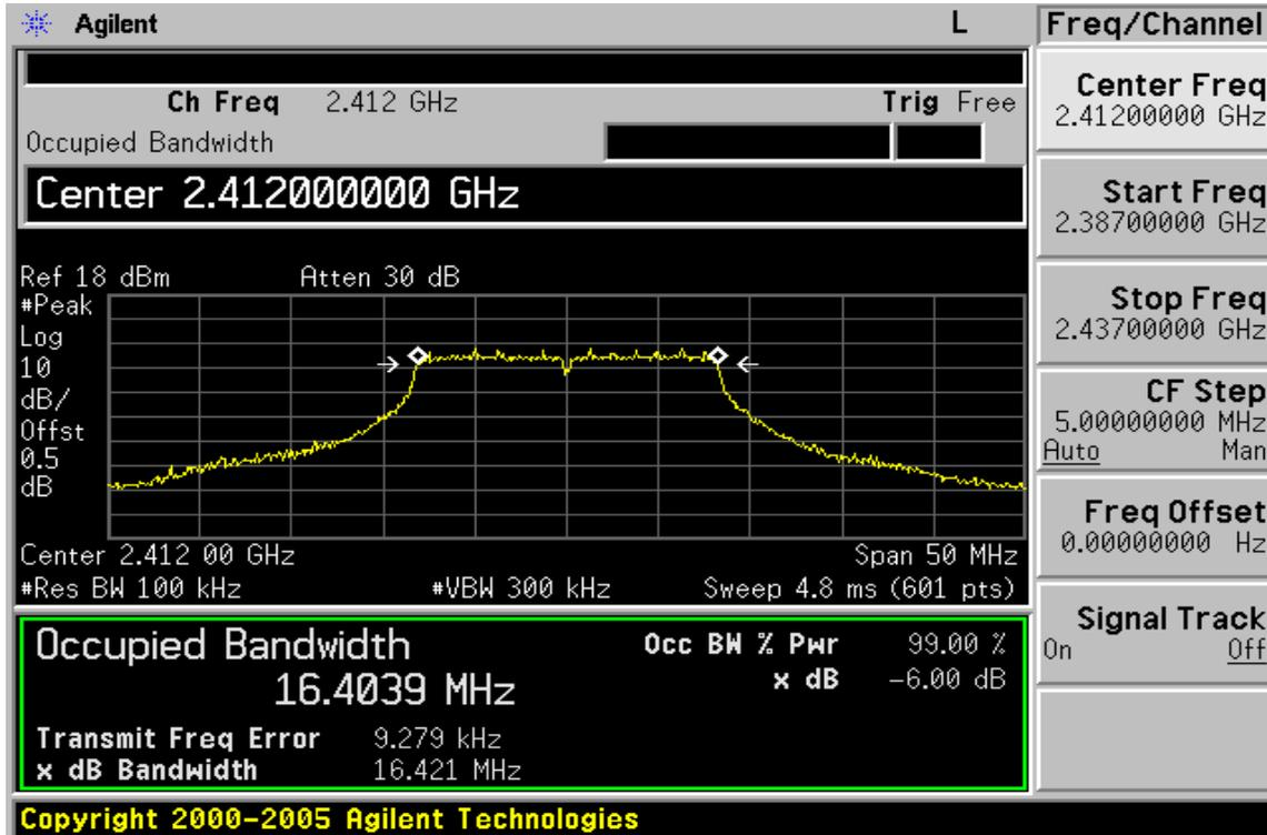
6dB Band Width Test Data CH-Mid
