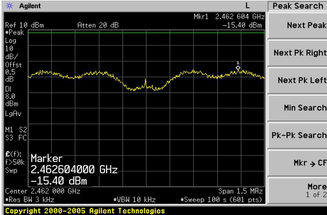
Power Spectral Density Test Plot (CH-Mid)
