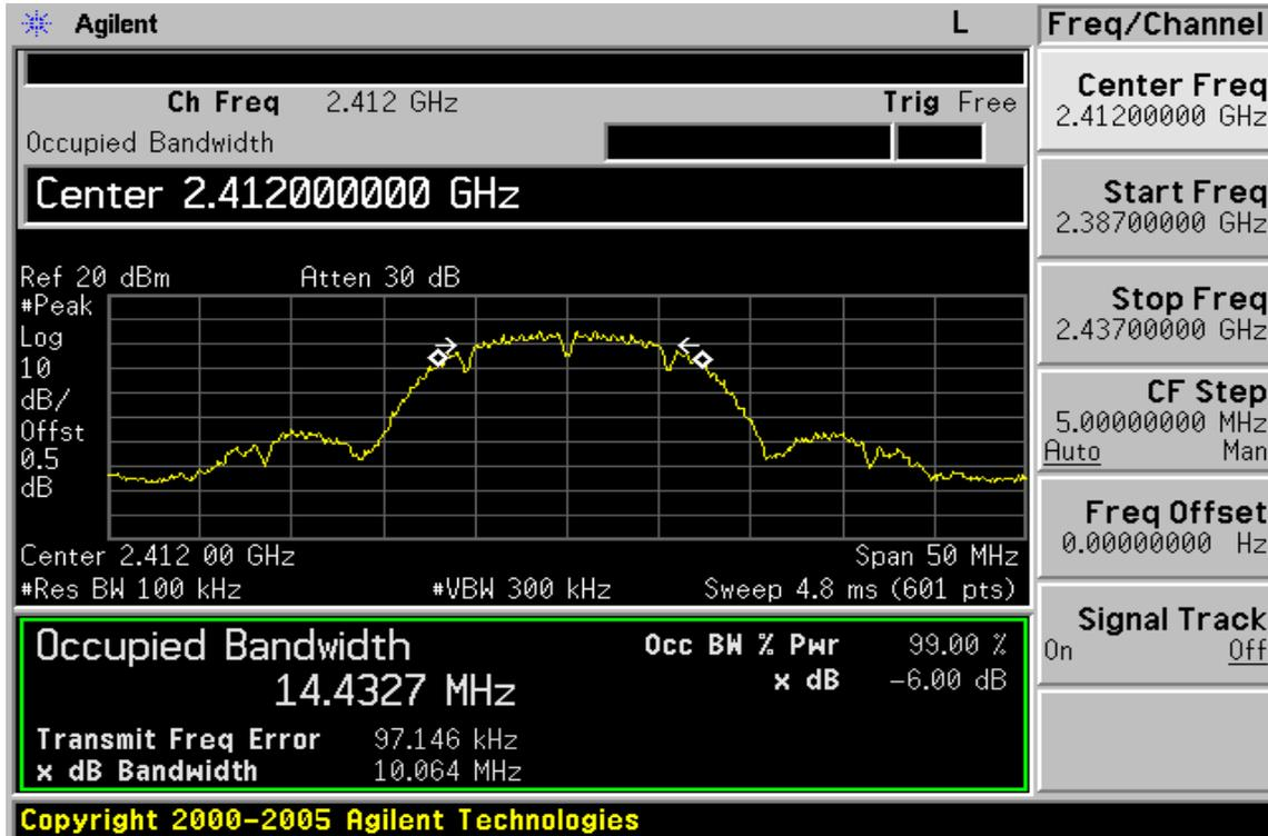
6dB Band Width Test Data CH-Mid
