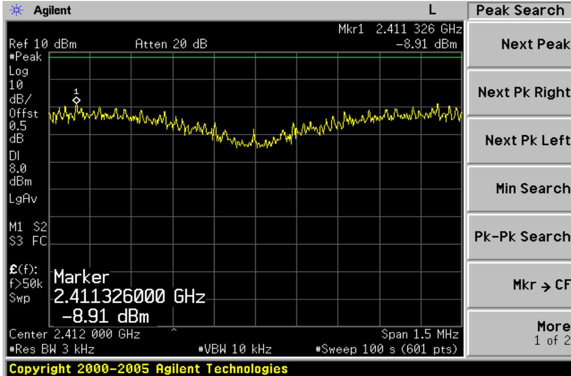
Power Spectral Density Test Plot (CH-Mid)
