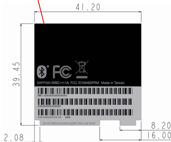
**NOTE: label on internal PCB board, not on back cover**
