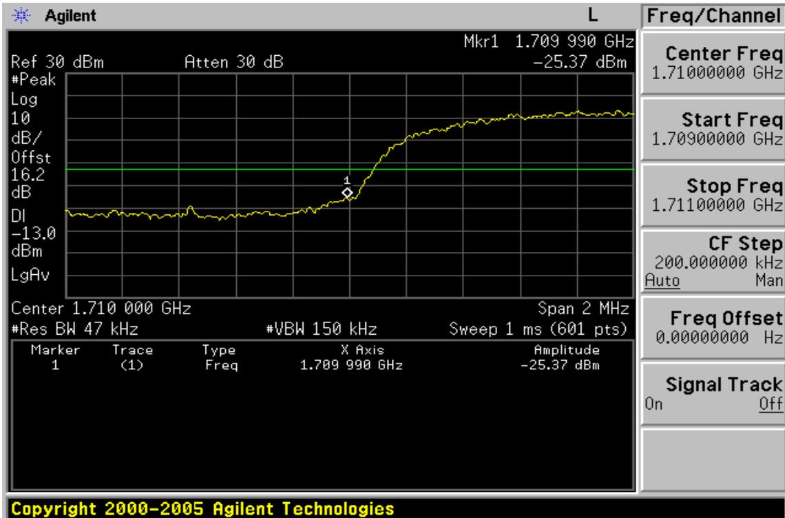
Figure 8-15: Band edge emission at antenna terminals –HSUPA IV Channel Highest
