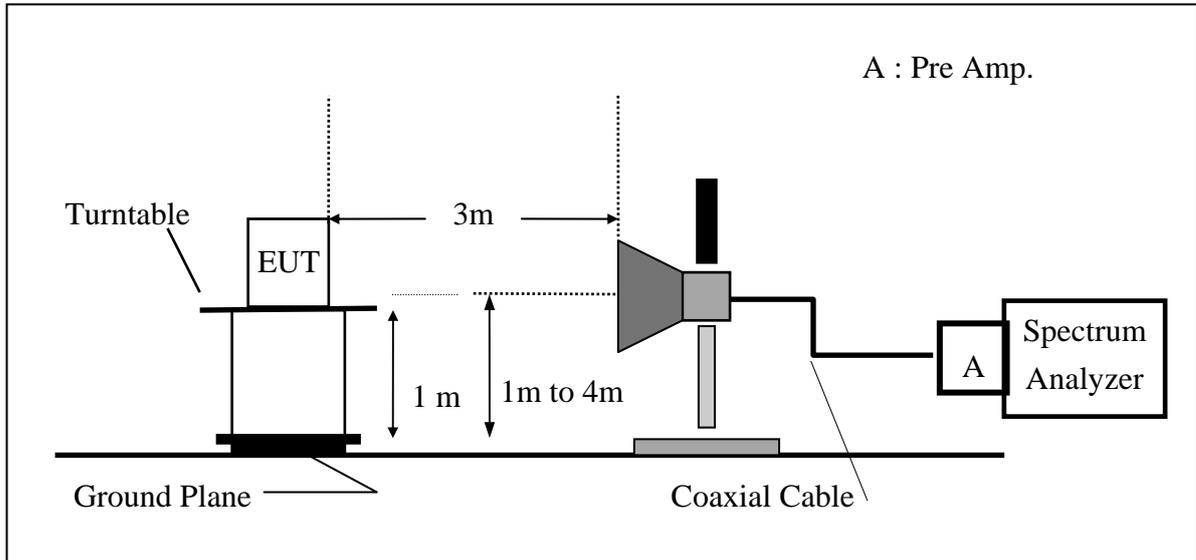
(C) Substituted Method Test Set-UP
