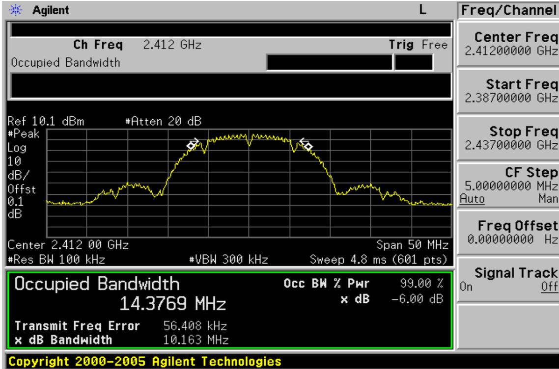
6dB Band Width Test Data CH-Mid
