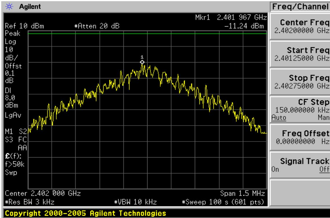
**Power Spectral Density Test Plot (CH-Mid)**
