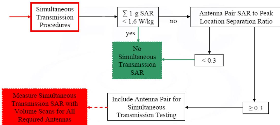
Fig. 3.1 KDB 648474 Simultaneous Transmission SAR Procedures for Handset Device
