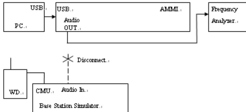
Figure 2: Signal Verification Setup
