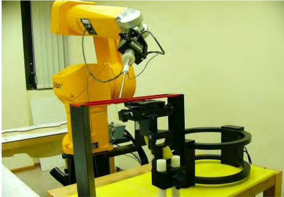
Fig.1 Photograph of the DASY 4 measurement System
