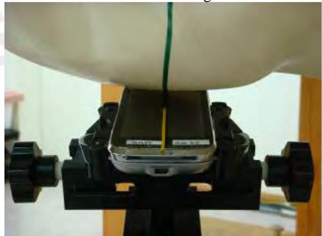
Fig.4 Right Head Section(Slider off)/ Ear-Tilt Position(15°)
