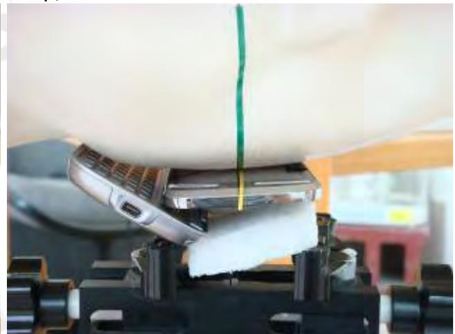
Fig.8 Left Head Section(Hold up) / Cheek-Touch Position
