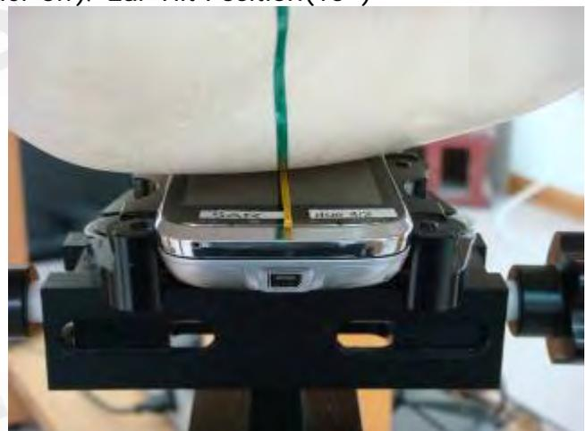
Fig.5 Left Head Section(Slider off) / Cheek-Touch Position
