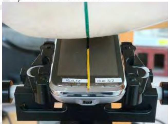
Fig.6 Left Head Section(Slider off) / Ear-Tilt Position(15°)
