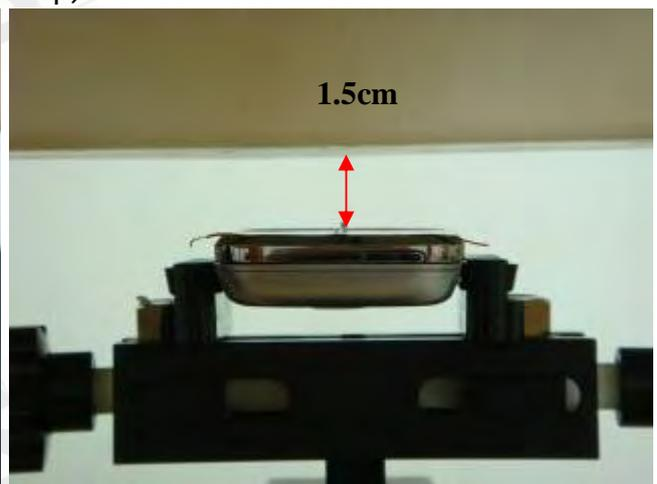
Fig.9 Body worn- EUT front to flat phantom and distance between flat phantom and mobile phone is 1.5 cm
