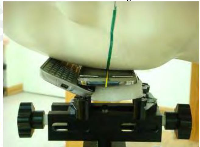
Fig.7 Right Head Section(Hold up) / Cheek-Touch Position
