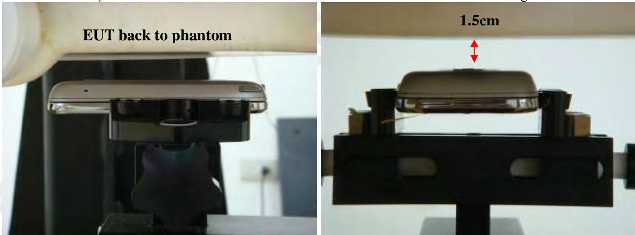
Fig.10 Body worn- EUT back to flat phantom and distance between flat phantom and mobile phone is 1.5 cm
