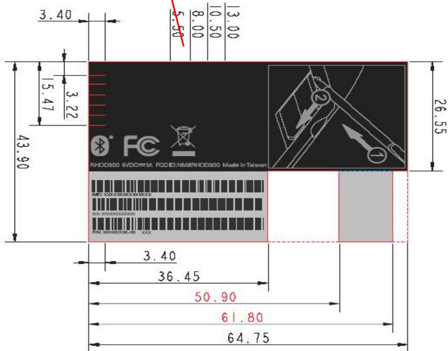
**NOTE: label on internal PCB board, not on back cover**
