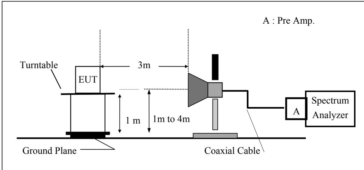
(C) Substituted Method Test Set-UP
