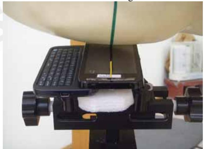
Fig.6 Right Head Section(Slider on)/ Ear-Tilt Position(15°)
