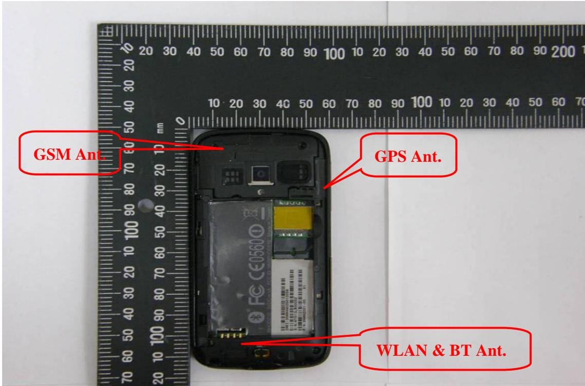
The min. distance is 9.2cm from GSM/WCDMA Antenna to WLAN/BT Antenna,
