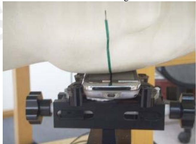
Fig.7 Left Head Section(Slider off) / Cheek-Touch Position
