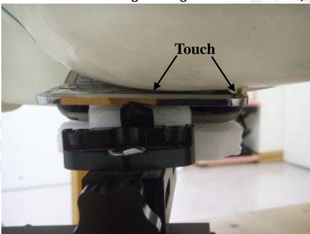
Fig.12 Left Head Section(Hold up) / Cheek-Touch Position
