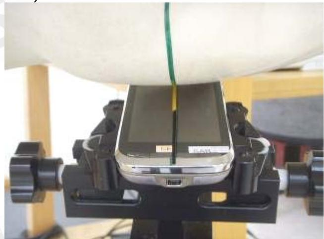
Fig.8 Left Head Section(Slider off) / Ear-Tilt Position(15°)
