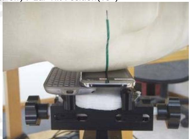
Fig.9 Left Head Section(Slider on) / Cheek-Touch Position
