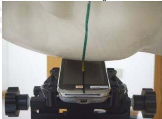
Fig.4 Right Head Section(Slider off)/ Ear-Tilt Position(15°)
