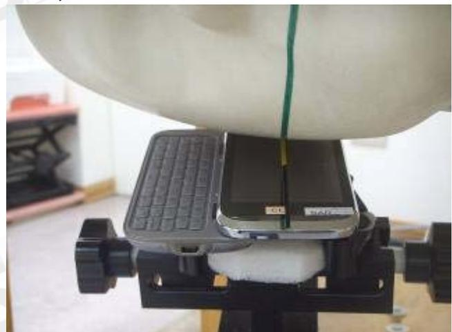
Fig.6 Right Head Section(Slider on)/ Ear-Tilt Position(15°)
