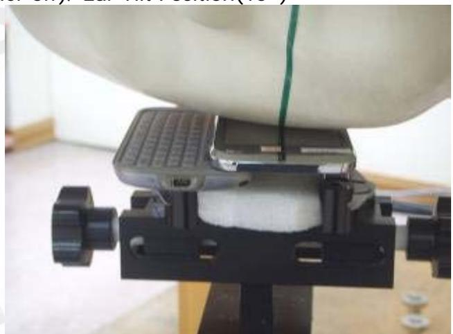
Fig.5 Right Head Section(Slider on) / Cheek-Touch Position
