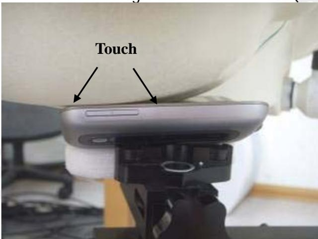
Fig.11 Right Head Section(Hold up) / Cheek-Touch Position
