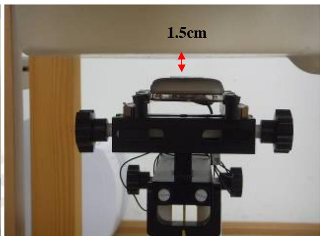
Fig.15 Body worn- EUT back to flat phantom and distance between flat phantom and mobile phone is 1.5 cm\_ repeated with headset
