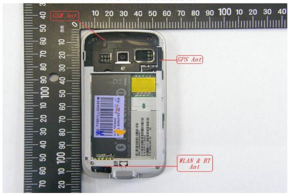
The min. distance is 8.5cm from GSM Antenna to WLAN/BT Antenna,
