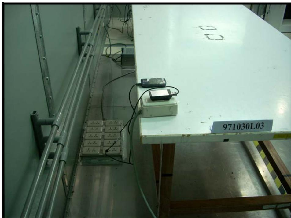
CONDUCTED EMISSION TEST (Test mode C)
