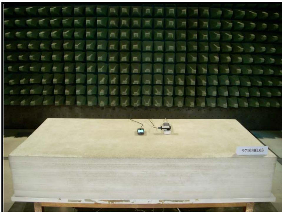
CONDUCTED EMISSION TEST (Test mode C)
