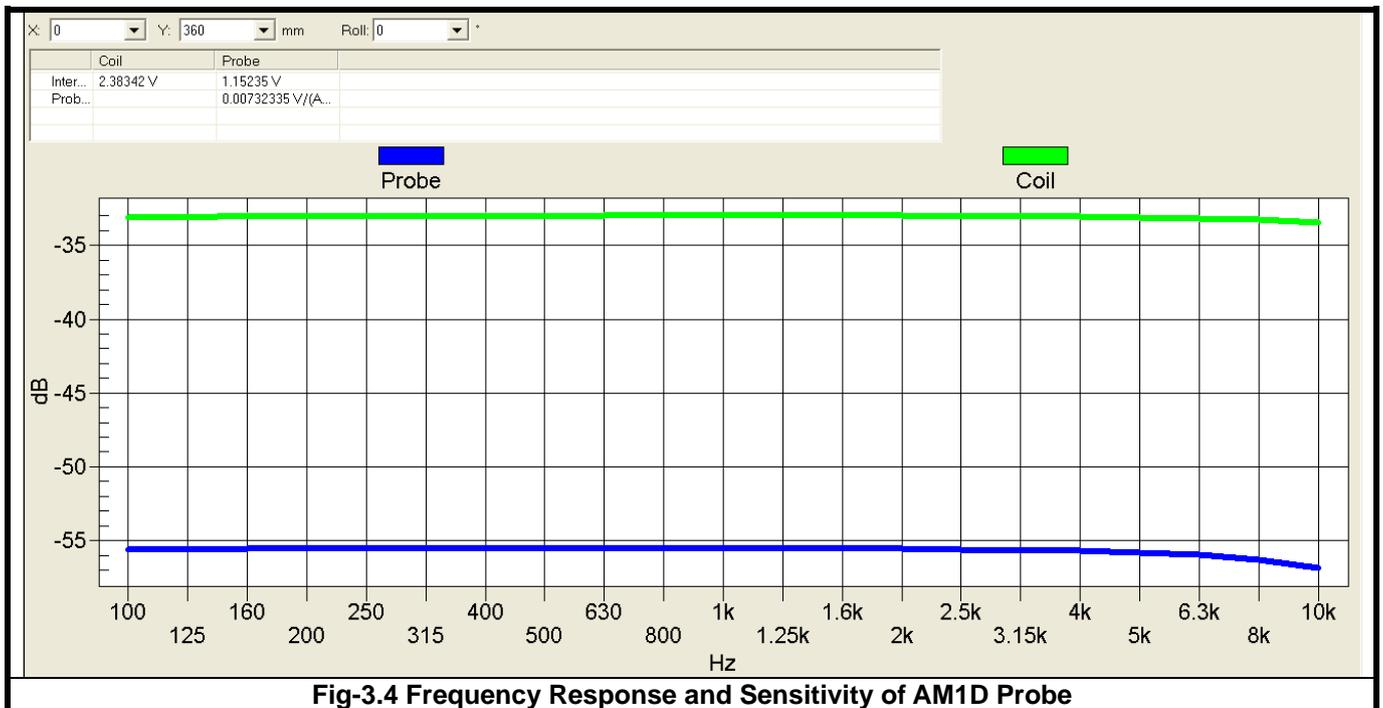
Fig-3.4 Frequency Response and Sensitivity of AM1D Probe
