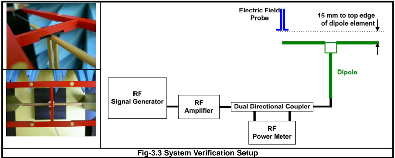
**Fig-3.3 System Verification Setup**
