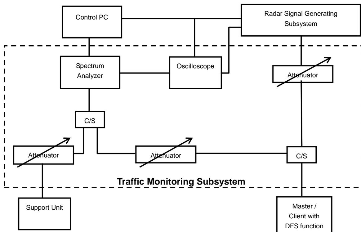
The test transmission will always be from the Master Device to the Client Device. While the Client device is set up to associate with the Master device and play the NTIA DFS MPEG file (6 ½ Magic Hours) from Master device, the designated MPEG test file and instructions are located at:
