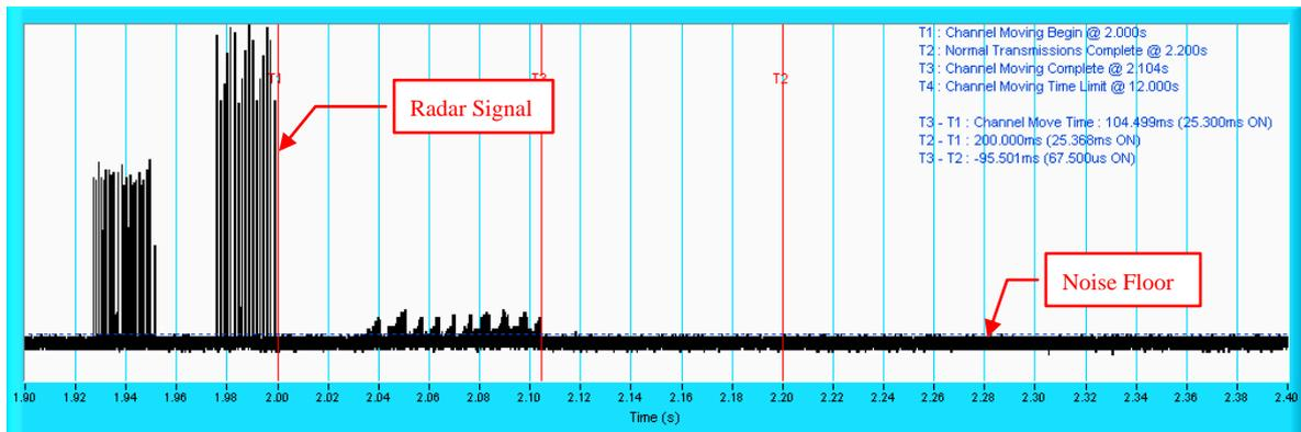
**NOTE:** An expanded plot for the device vacates the channel in the required 500ms.
