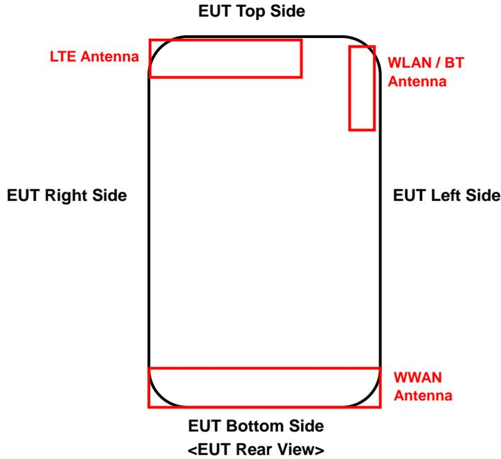
The separation distance for antenna to edge:
