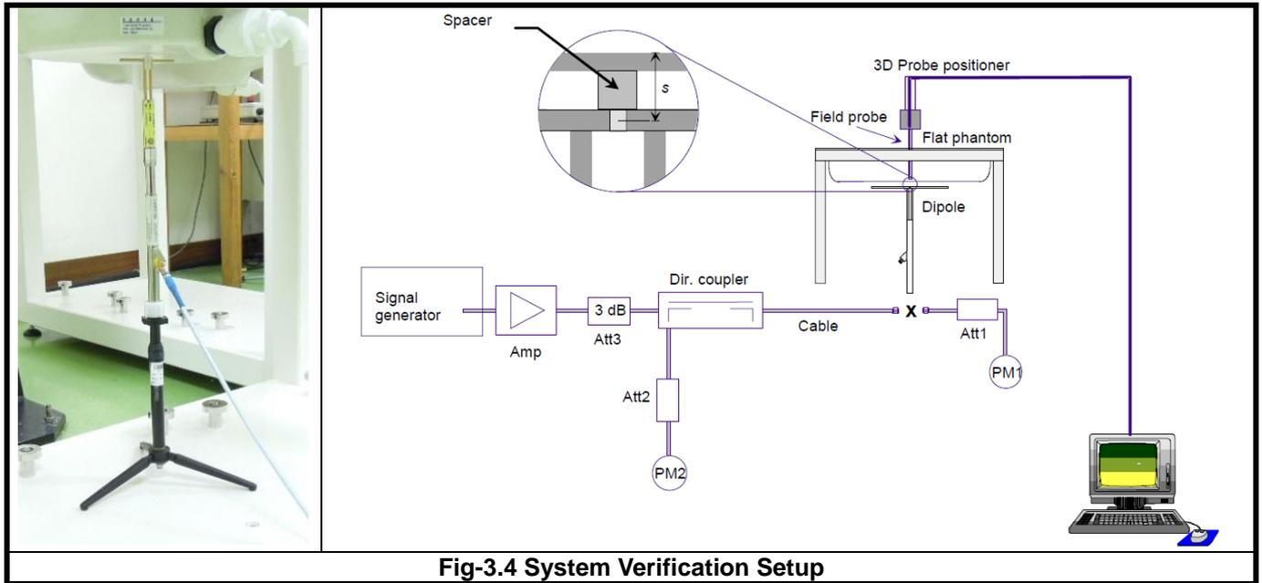
**Fig-3.4 System Verification Setup**
