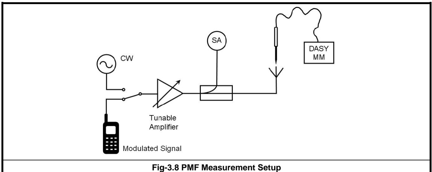
**Fig-3.8 PMF Measurement Setup**
