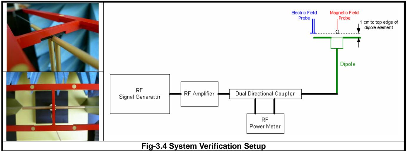
The validation dipole is placed beneath the center of arch phantom. The power meter measures the forward power at the location of the system check dipole connector. The signal generator is adjusted for the desired forward power, 100 mW (20 dBm) at the dipole connector and the RF power meter is read at that level. After connecting the cable to the dipole, the signal generator is readjusted for the same reading at RF power meter.
