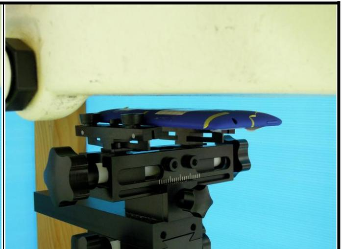
Rear Face of EUT with 1.0 cm Gap
