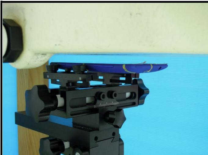
Front Face of EUT with 1.0 cm Gap
