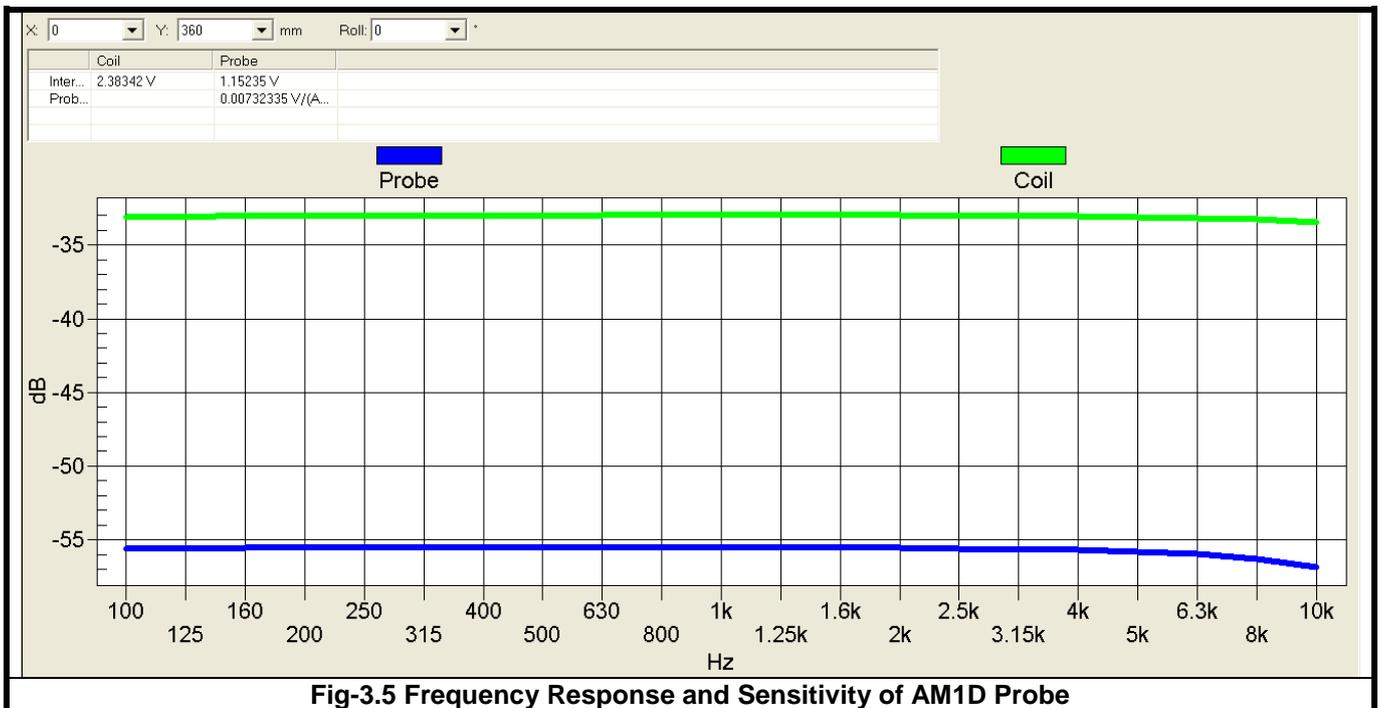
**Fig-3.5 Frequency Response and Sensitivity of AM1D Probe**
