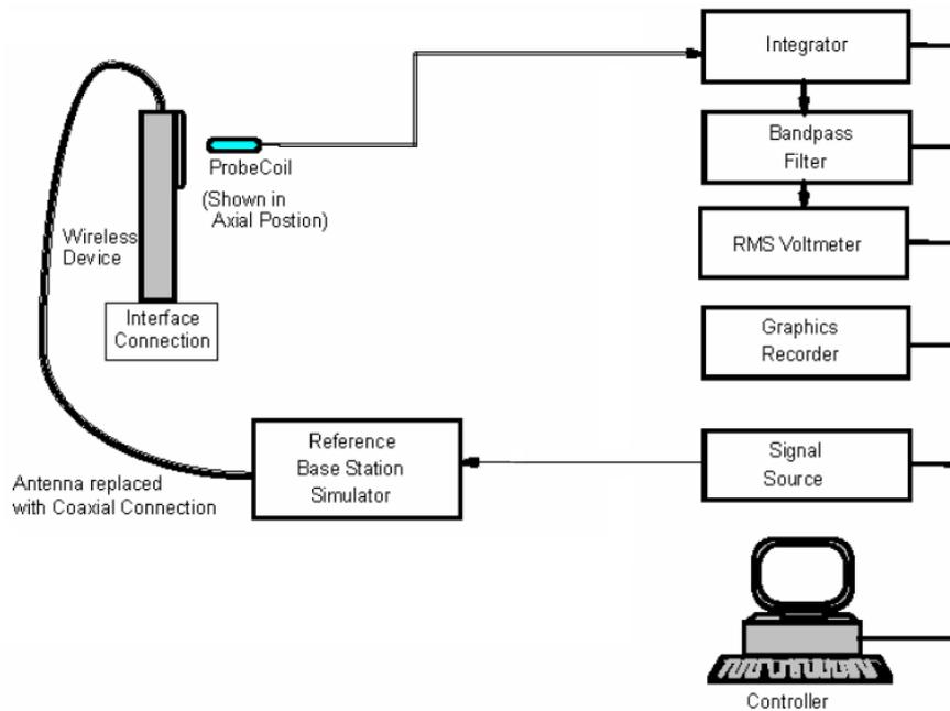
**Fig-3.7 T-Coil Measurement Test Setup**
