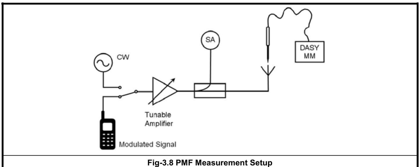
Fig-3.8 PMF Measurement Setup
