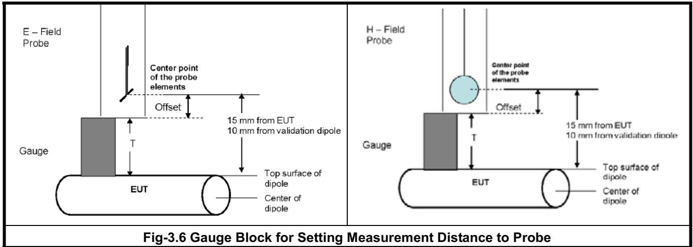
**Fig-3.6 Gauge Block for Setting Measurement Distance to Probe**
