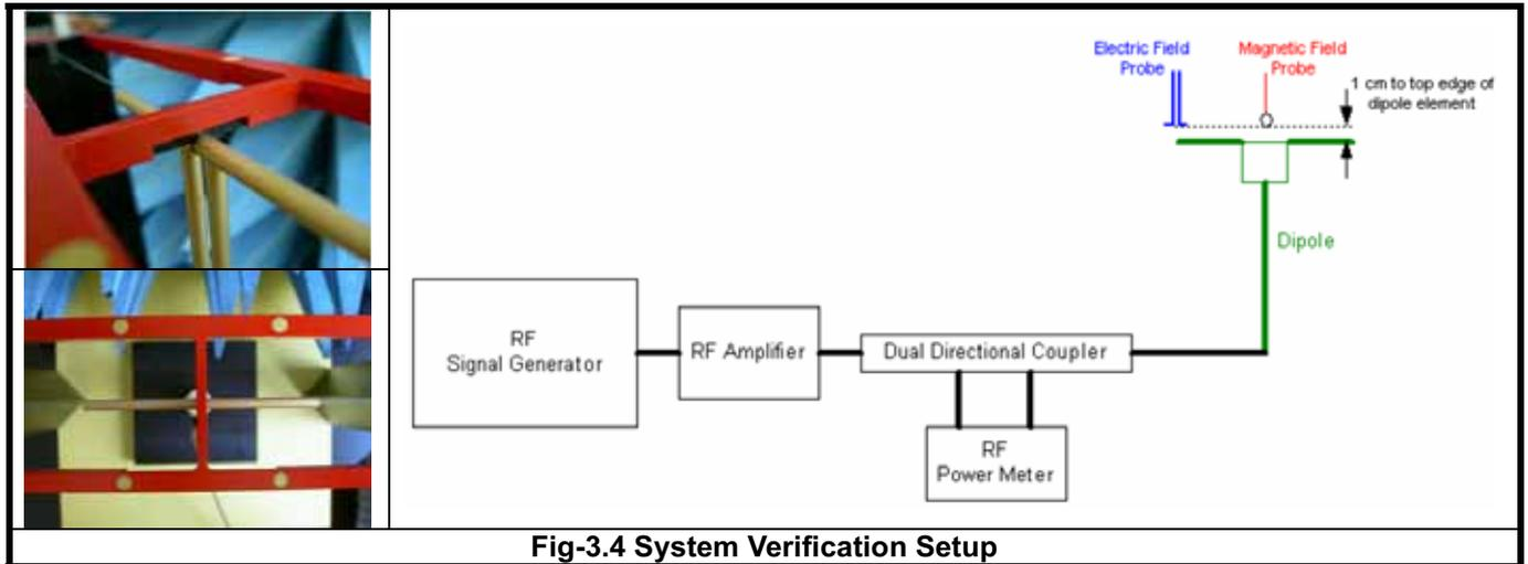
**Fig-3.4 System Verification Setup**
