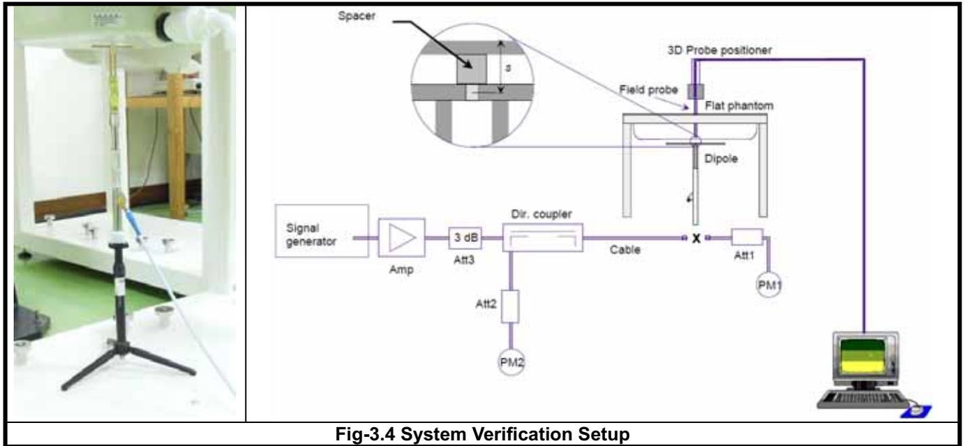
Fig-3.4 System Verification Setup
