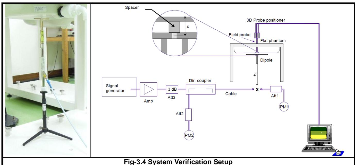
**Fig-3.4 System Verification Setup**
