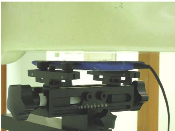
**Front Face of EUT with 1 cm Gap
