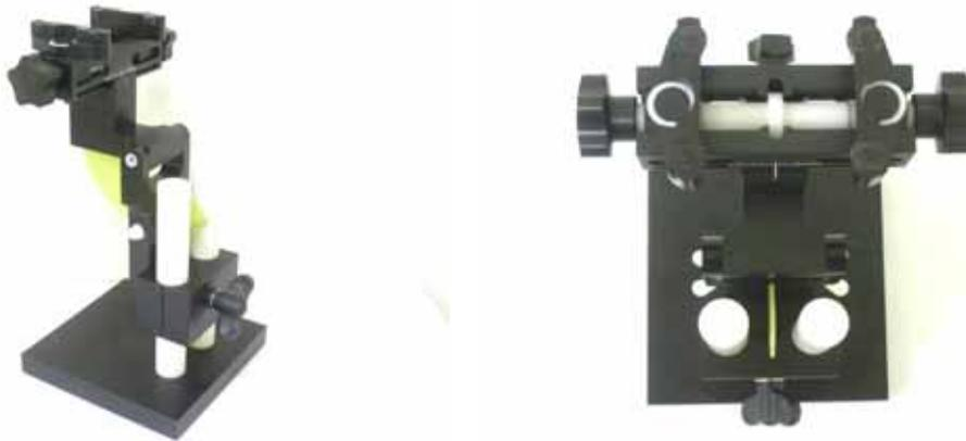
**CONSTRUCTION** Supports accurate and reliable positioning of any phone effect on near field  $\pm 0.5\text{dB}$
