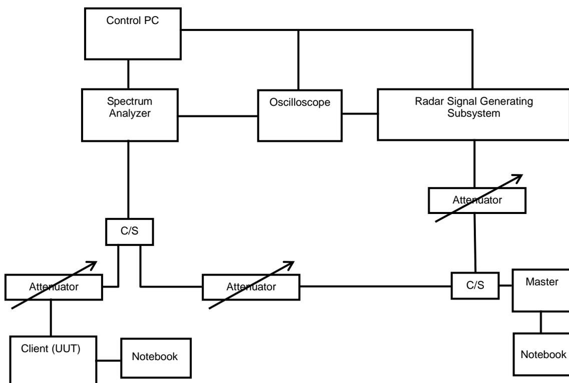
The UUT is a U-NII Device operating in Client mode without radar detection. The radar test signals are injected into the Master Device.
