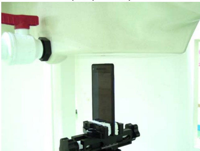
Top Side of EUT with 1 cm Gap (Hotspot Mode)
