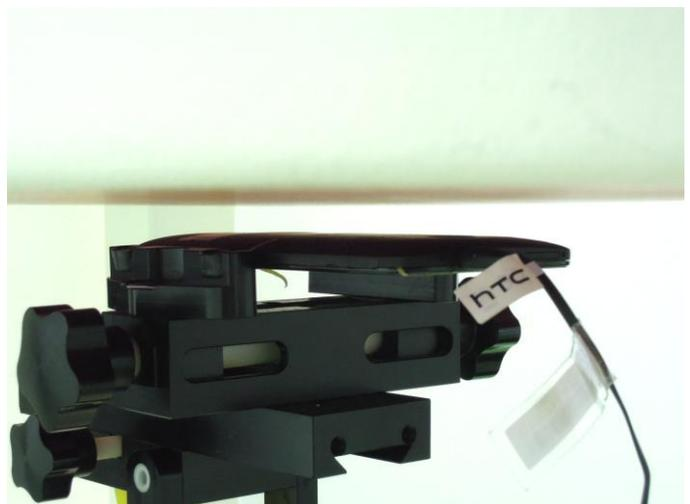
Rear Face of EUT with 1 cm Gap
