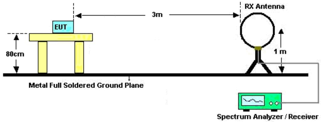
For radiated emissions from 30MHz to 1GHz
