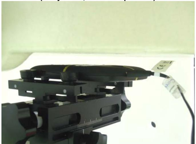
**Rear Face of DUT with 1 cm Gap
