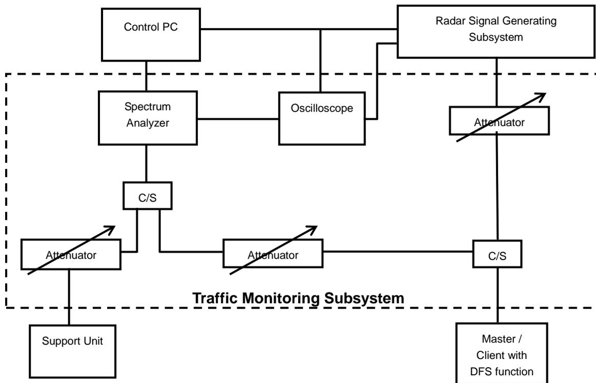
The test transmission will always be from the Master Device to the Client Device. While the Client device is set up to associate with the Master device and play the 5\_GHz\_Audio\_Test\_file.wav from Master device, the designated wav test file and instructions are located at:
