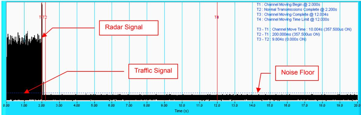
**NOTE:** T1 denotes the start of Channel Move Time upon the end of the last Radar burst. T2 denotes the data transmission time of 200ms from T1. T3 denotes the end of Channel Move Time. T4 denotes the 10 second from T1 to observe the aggregate duration of transmissions.
