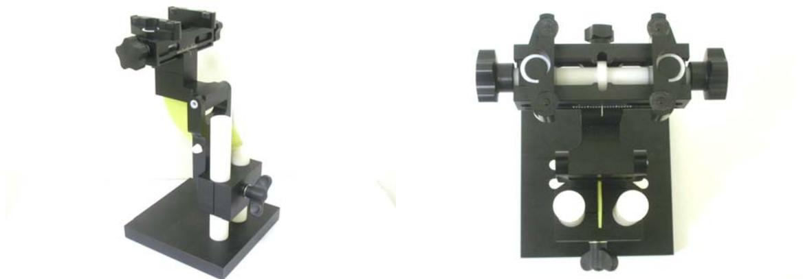
**CONSTRUCTION** Supports accurate and reliable positioning of any phone effect on near field  $\pm 0.5\text{dB}$
