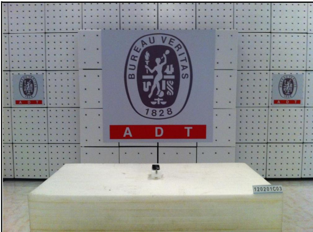
Charging mode for all radiated emission test
