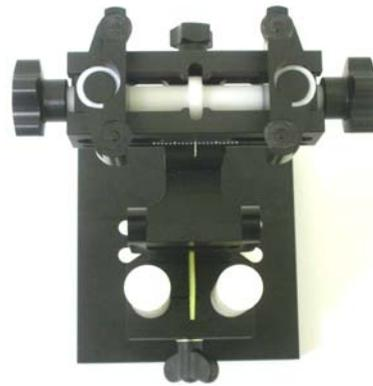
**CONSTRUCTION** Supports accurate and reliable positioning of any phone effect on near field  $\pm 0.5\text{dB}$
