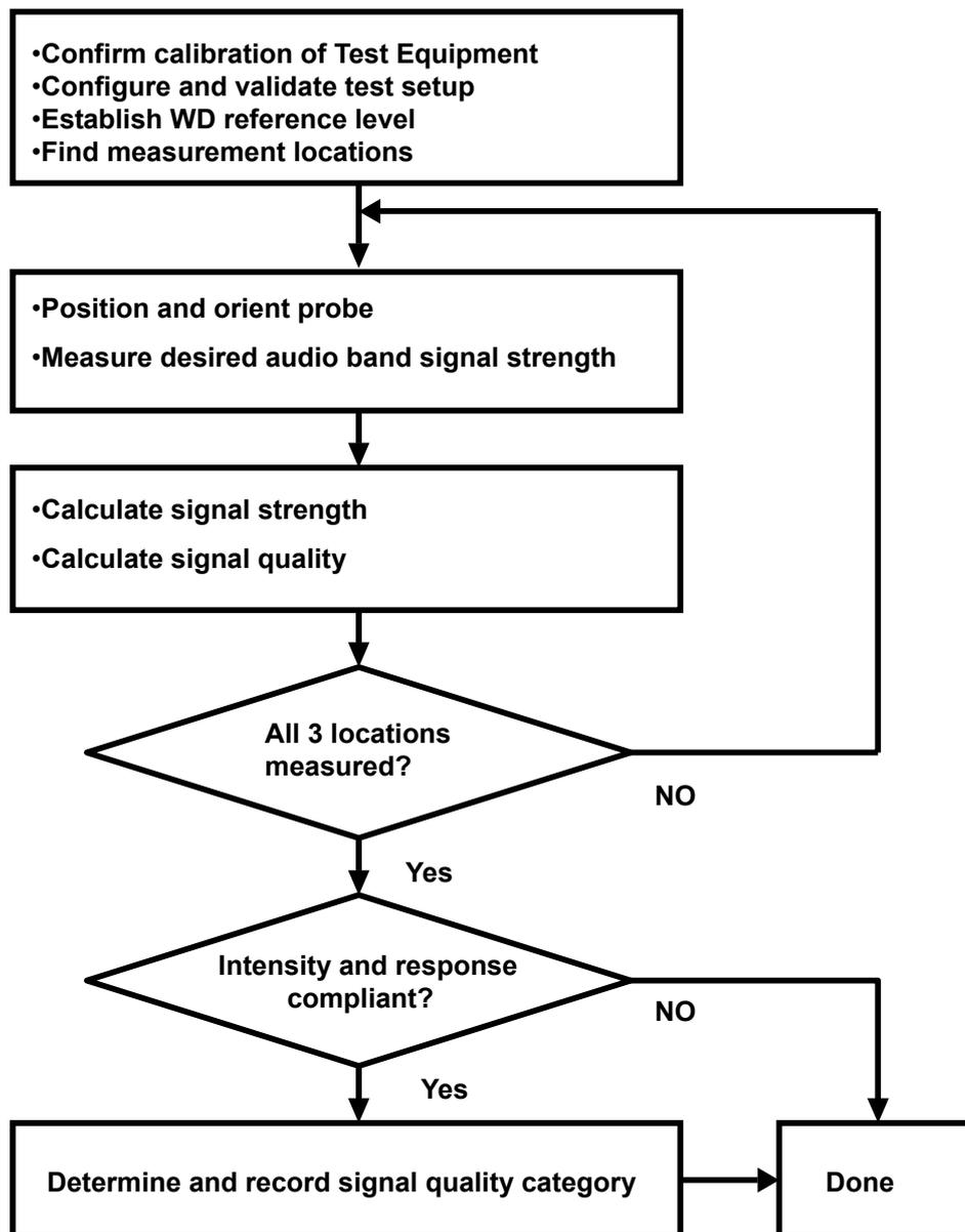
The following steps were a typical test scan for the wireless communications device:
