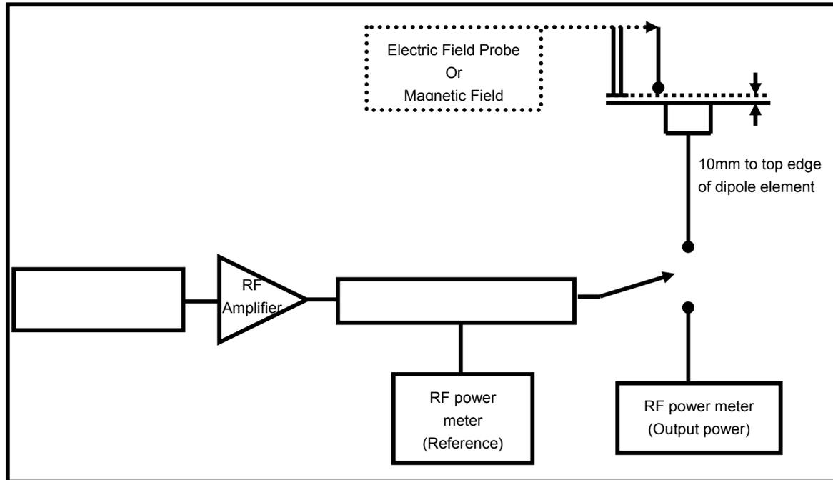
2. The dipole was energized with a 20dBm un-modulated continuous-wave signal.
