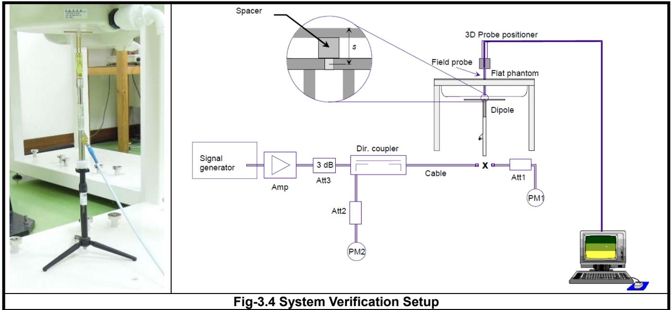
**Fig-3.4 System Verification Setup**
