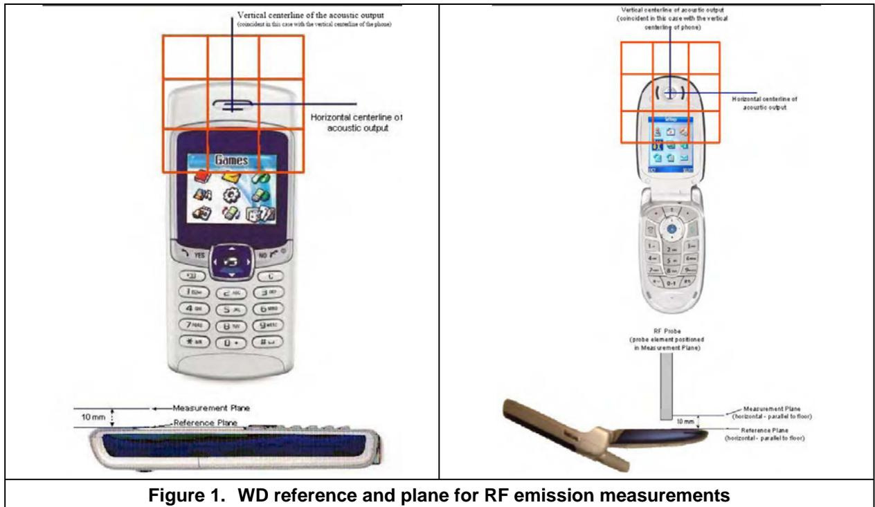
**Figure 1. WD reference and plane for RF emission measurements**
