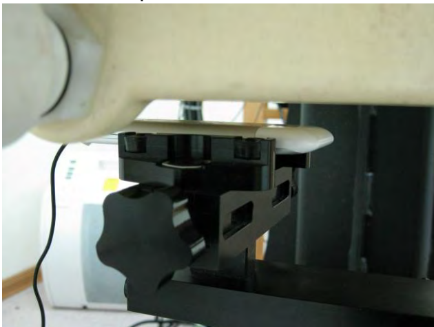
Fig.12 Hotspot mode- EUT Back to flat phantom and distance between flat phantom and mobile phone is 1 cm_ repeated with Headset.
