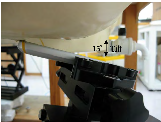
Fig.4 Right Head Section / Ear-Tilt Position(15°)
