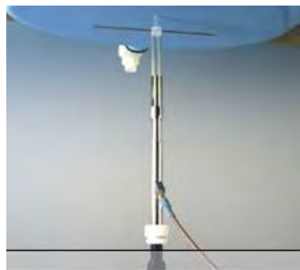
Photograph of the dipole Antenna
