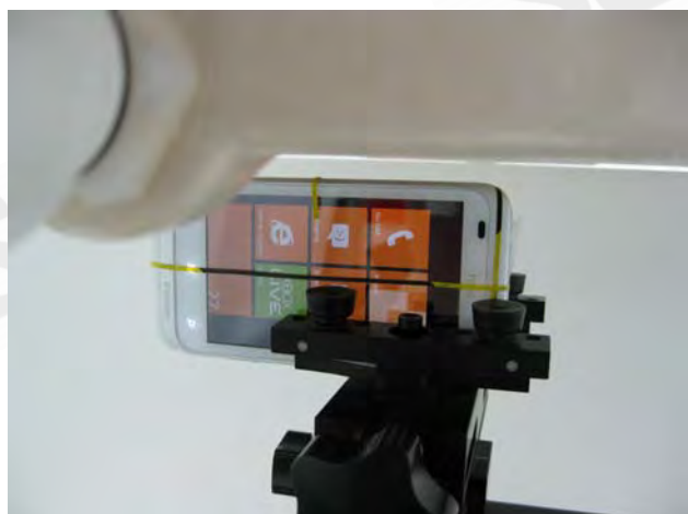
Fig.12 Hotspot mode- EUT Left to flat phantom and distance between flat phantom and mobile phone is 1 cm.
