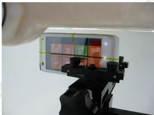
Fig.11 Hotspot mode- EUT Right to flat phantom and distance between flat phantom and mobile phone is 1 cm.
