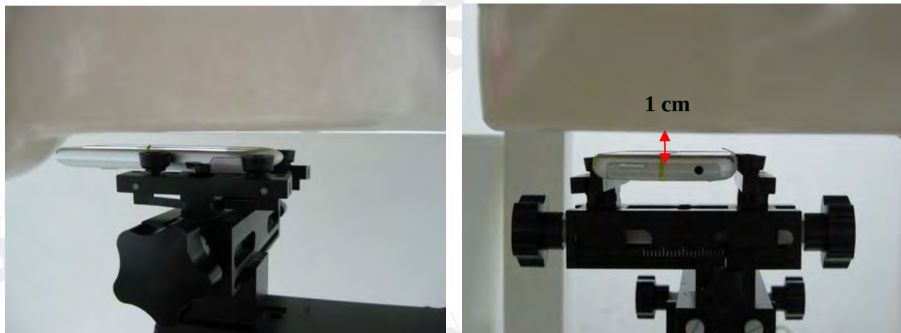
Fig.7 Hotspot mode- EUT front to flat phantom and distance between flat phantom and mobile phone is 1 cm.
