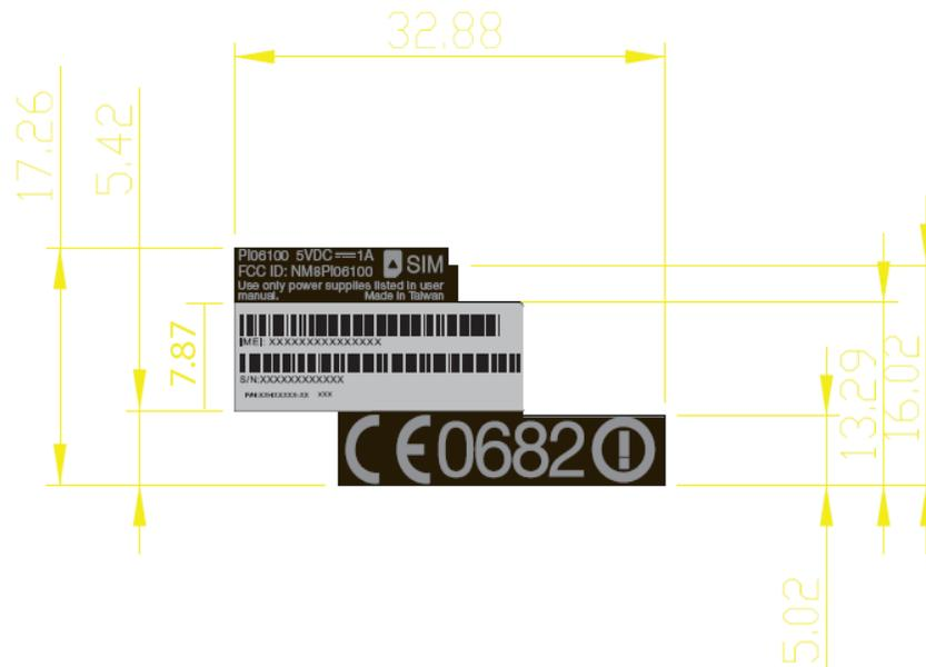
**NOTE: Label on internal PCB board, not on back cover**
