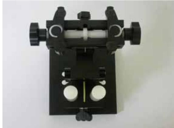
**CONSTRUCTION** Supports accurate and reliable positioning of any phone effect on near field  $\pm 0.5\text{dB}$
