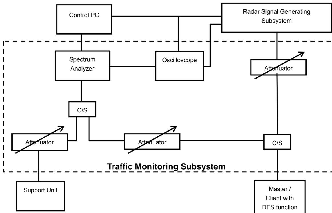
The test transmission will always be from the Master Device to the Client Device. While the Client device is set up to associate with the Master device and play the Audio file 5\_GHz\_Audio\_Test\_file.wav from Master device, the designated Audio test file and instructions are located at: <http://ntiacsd.ntia.doc.gov/dfs/>.
