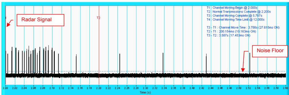
**NOTE:** Room-in of the first 600ms after radar signal applied.
